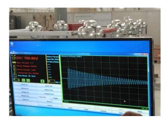
**CDS Series turn-to-turn overvoltage test system** is performed by repeatedly charging a capacitor and discharging it, through sphere gaps, into the reactor windings. The type of overvoltage that the reactor is subjected to is similar to a switching impulse with an exponentially decaying sinusoidal wave shape.
