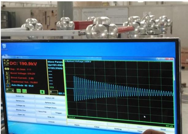
**CDS Series turn-to-turn overvoltage test system** is performed by repeatedly charging a capacitor and discharging it, through sphere gaps, into the reactor windings. The type of overvoltage that the reactor is subjected to is similar to a switching impulse with an exponentially decaying sinusoidal wave shape.
