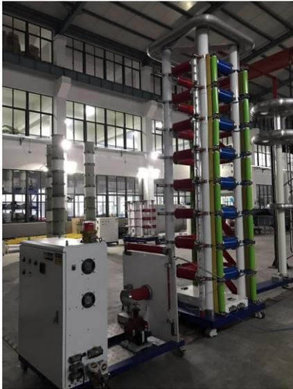
**CDYQ series Impulse Voltage Test System** is design as Q structure, it can be used to generate impulse voltage what simulate lightning strokes (LI: 1.2/50us) and switching surges (SI: 250/2500us). The total charging voltage range is from 200kV-4800kV with stage energy of 5 to 40kJ. Applications covered include testing according to IEC, ANSI/IEEE/GB as well as other national standards.
