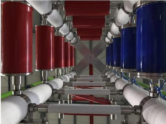
**CDYQ Series Impulse Generator** is the main part of the impulse voltage test system. Four epoxy glass support hangs on two capacitors each stage, constituting a stable components structure for the whole impulse voltage generator. The impulse generator has 2-24 stages, constituting a tower form structure, each stage is a cascade connection, disassembly and maintenance are convenient, and the whole structure is stable.
