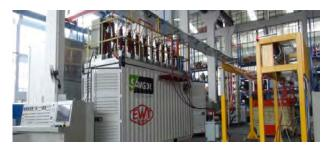
**5MVA Automatic Distribution Transformer Test System**
