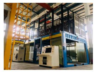
5MVA Automatic Distribution Transformer Test System
