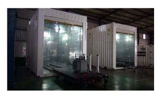
Module Type Shielding Room for PD Measurement
