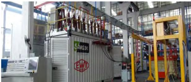
**5MVA Automatic Distribution Transformer Test System**
