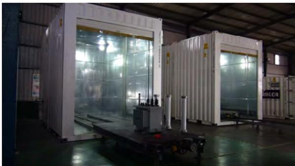
**Module Type Shielding Room for PD Measurement**
