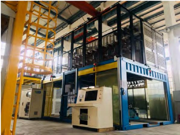
5MVA Automatic Distribution Transformer Test System
