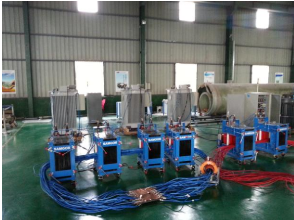
220kV 7000A Cable Heat Cycle Test System
