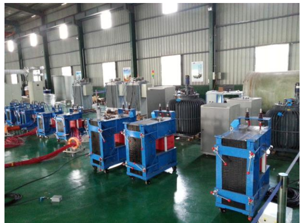
220kV 5000A Cable Heat Cycle Test System
