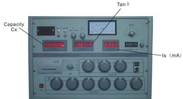
The socket connecting the standard capacitor and measured sample is on the back of this apparatus. There are totally two earthed terminals on the front and back. The external connection is shielded cable. The capacitor cabinet is electrostatic shielding type to prevent from interference.
