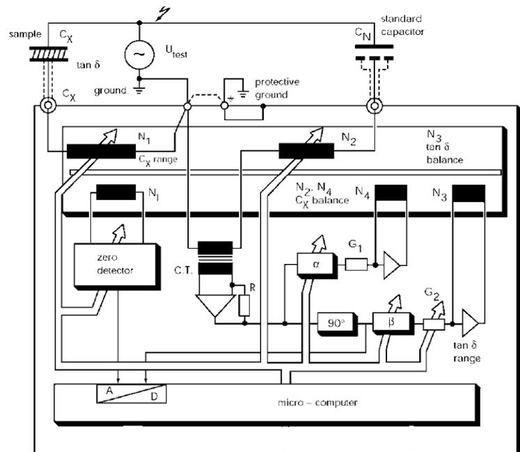
Control of the reference parameters (number of turns, fine balance current,  $\tan\delta$ , balance current, measurement range) is achieved by the microcomputer based upon data supplied by the zero detectors. At the end of the balancing cycle the actual values for  $C_X$   $\tan$  and test voltage are calculated from the reference parameters and displayed.
