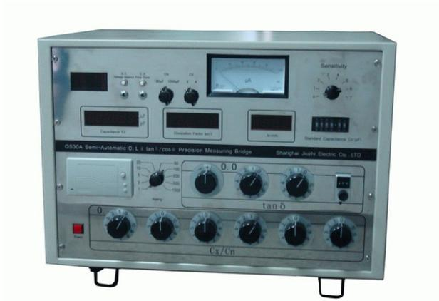
The measuring system type **QS30A** is designed for determining the capacitance and dielectric dissipation factor of liquid and solid insulants, cables, capacitors, line transformers, generators, motors, bushings etc. Furthermore it can also be used for power loss measurement on shunt reactors or similar apparatus. This system is suitable for both low and high voltage measurement at line frequency.
