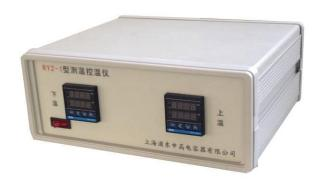
This temperature control unit is used to heat and to control the desired temperature of the solid insulants test cell, type RY2.
