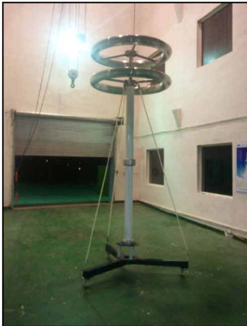
900kV Resistive Voltage Divider (10ohm)
