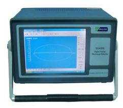
SG4008 multi-channel digital partial discharge measuring system developed by SAMGOR up to minutes, which have powerful anti-interference capability and up to six channels. It can collect data from single to six channels and show in the windows in the same time.
