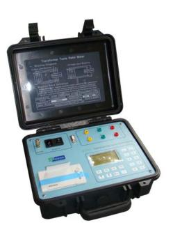
SG7001 is an important basic measurement for power transformer diagnosis. It helps to detect faulty transformer windings as well as defective tap changer positions. This advanced instrument automatically recognizes winding connections and vector group numbers of transformer windings. Just connect the measuring cables and press the start button and get the test results.
