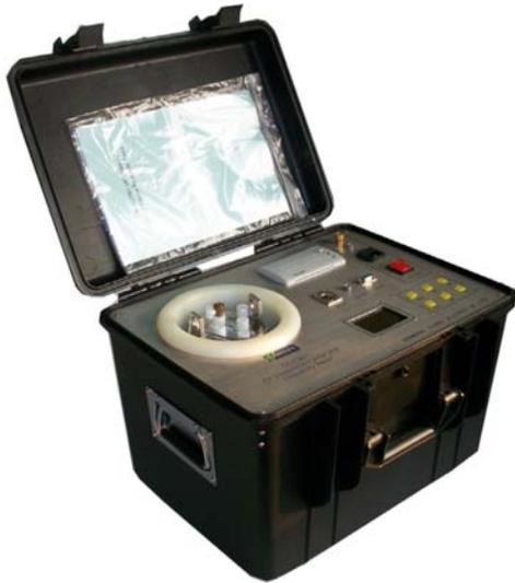
SG7501 Oil Dissipation Factor and Resistivity Meter is used to measure dissipation factor, dielectric constant and resistivity for oil. The set is all-in-one structure, with internal oil cup, temperature control, AC bridge, high resistance meter, AC/DC test voltage and standard capacitor etc.
