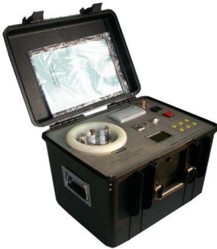
SG7501 Oil Dissipation Factor and Resistivity Meter is used to measure dissipation factor, dielectric constant and resistivity for oil. The set is all-in-one structure, with internal oil cup, temperature control, AC bridge, high resistance meter, AC/DC test voltage and standard capacitor etc.
