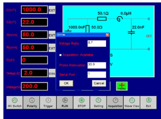
**Advanced Analysis Capability** Fine adjust all parameters in the major loop, more than 10,000 steps available for charging capacitor ( $C_1$ ), load capacitor ( $C_2$ ) front wave resistor ( $R_f$ ) and tail wave resistor ( $R_t$ ), more than 35 steps available for inductor; Hundred times more choice for parameters and high resolution and accuracy digital analyzer make the advanced analysis be a easy and sample work.
