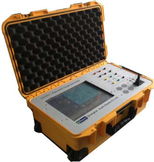
SG7601/SG7602 Digital Recurrent Surge Generator is the first digital and most big range recurrent surge generator, it is a low voltage equivalent, with one stage only, it has wide range of applications includes the testing of models, the study of voltage distribution in high voltage windings during impulse voltage stresses and the predetermination of the impulse circuit parameters of the test plants.
