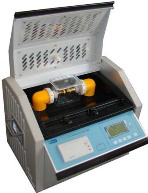
For many electric equipments used in power system and enterprises, inner insulation is mostly oil-insulated. Oil dielectric strength test is one of the essential routine tests. SG7808 Oil Dielectric Test Set is the ideal testing device for oil dielectric strength. The test sets are fully automatic.
