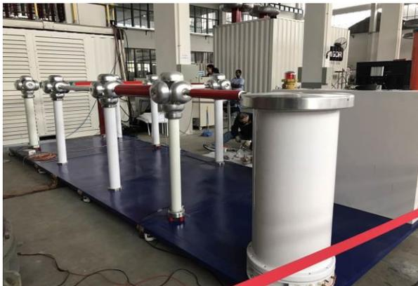
**The high voltage modular AC/DC/Impulse test system** is design to be used to test up to 200kV AC voltage, 260kV DC voltage, 240kV LI and 200kV SI. This modular test system is available in a variety of configurations and can be easily expanded at a later date.
