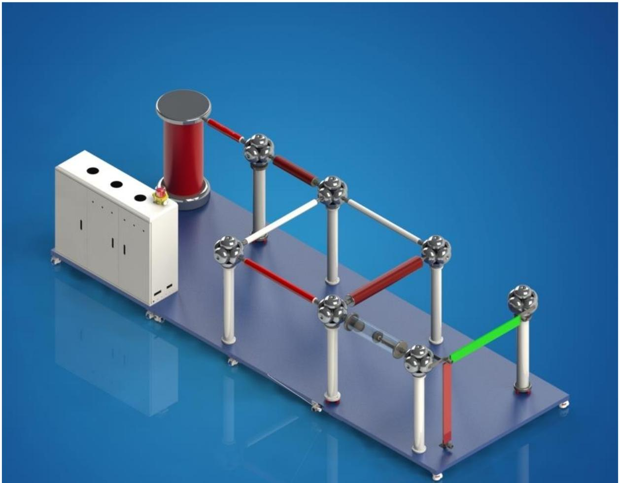
**Typical 100kV AC / 250kV DC / 250kV LI-SI / 250kV LIC Block Diagram:**
