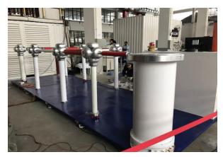
The high voltage modular AC/DC/Impulse test system is design to be used to test up to 200kV AC voltage, 260kV DC voltage, 240kV LI and 200kV SI. This modular test system is available in a variety of configurations and can be easily expanded at a later date.
