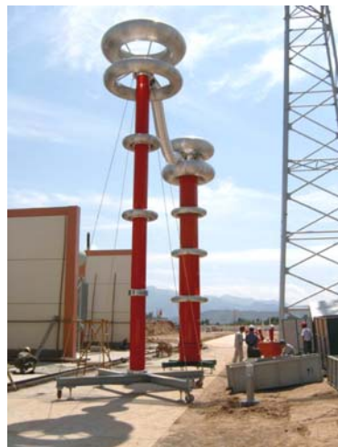
1000KV/5A Module Tunable Frequency Resonant Test System (Oil Type)
