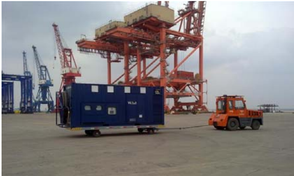
3000kVA 60Hz Port Shore Power Source
