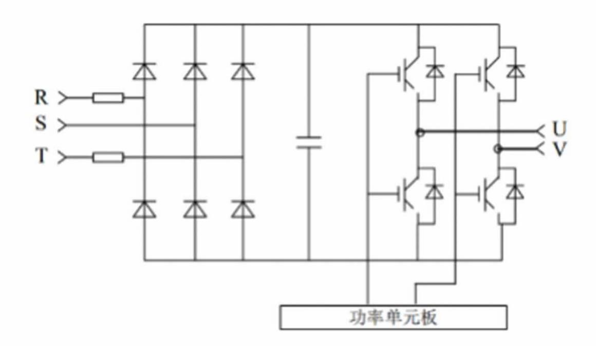
The basic structure of power unit is AC-DC-AC, three-phase full bridge rectifying input, and single-phase H bridge converting output. DC charging section make AC three-phase power to change to DC power and it is stored in the capacitor module to be a stable DC source. The converting bridge by the IGBT module can generate the sine waveform single phase AC power by PWM control.
