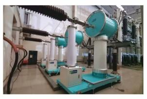
measurement tap is changing at its secondary side and the software can adjust the measurement range in automatic way. Such method makes the test much simple and more efficient since the engineer need not to change the tap in the primary side for each test section.
