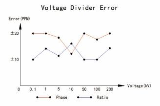
Loss measurement: The voltage and current from three sets of HV electronic voltage dividers and current transformers will be delivered to the power analyzer of NORMA 5000 or WT5000. All the data will be processed by the analyzer including voltage, current, loss, frequency, power factor, harmonic, and waveform. The loss measurement accuracy will be different with the power factor value. The accuracy will be less than 1.15% at very lower power factor of 0.008.
