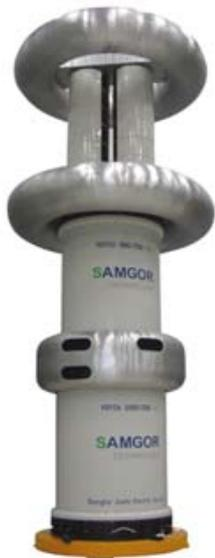
Conventional AC test transformers are especially designed for testing objects of medium capacitance in the factory. These systems are particularly suited for tests requiring stable voltage even if the load changes during the testing (heavy corona, wet & pollution tests) or when the load is of inductive kind (inductive voltage transformers). The possibility to stack several of these transformers allows reaching very high voltages by keeping a reasonable floor space.
