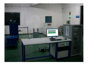
Over Voltage Cycle Test System is the type test, repeated over voltage from lowest rated temperature to the ambient temperature to improve the dielectric performance for the shunt capacitor above 10kV. In the recent year, this test is more popular to done in the modern factory.
