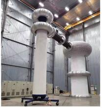
YL series High Voltage Standard Capacitor has unique internal voltage distribution structure, which allows the whole capacitor to work continuously at full rated voltage with the humidity of 95%. Equipped with composite outskirt, YL standard capacitor can work outdoor. The good 304 stainless steel is applied as the electrode for the capacitor so as to ensure the high stability, low temperature coefficient and low
