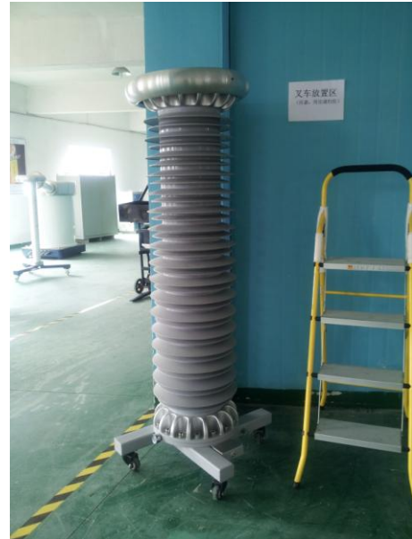
YL400kV/10pF Standard Capacitor (Outside Use)
